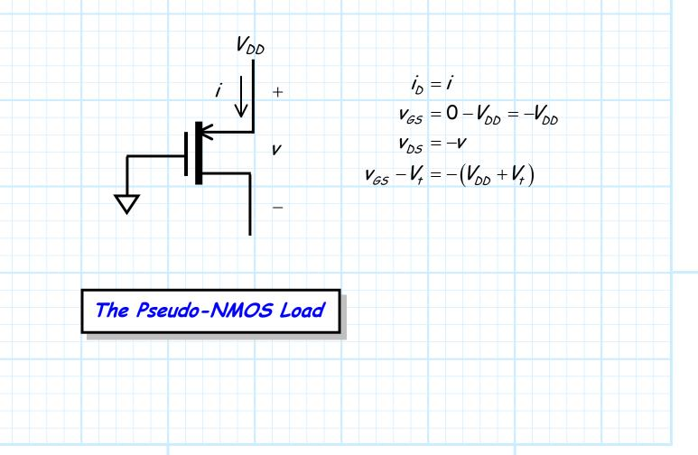
Note that  $v_{GS} = -V_{DD} < V_t$ , so that the load is **not** in cutoff—it can either be in **saturation or triode**.
