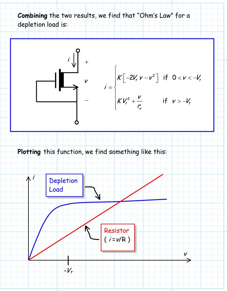
Note that the behavior of a Depletion Load and a resistor are **very different**—however they are precisely the **same** in two key ways:
